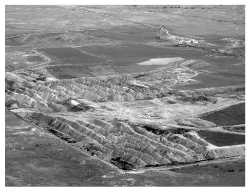
Ridges of mine spoil stand 12 deep at the Coal Creek Mine, operated by Arch Coal, near Wright, Wyo. Spoil ridges must be reshaped by bulldozers to create final surface grade before topsoil can be replaced and vegetation regrown. Because a significant amount of mine reclamation must be deferred until the mine ceases production, there will be lots of reclamation work that could extend the careers of coal miners.
