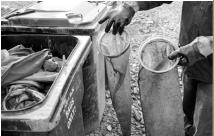
Filter socks collect and condense sludge and pipe scale, hard and insoluble deposits, resulting in a highly concentrated radioactivity level. Filter socks have been illegally dumped in the North Dakota communities of Watford City, Noonan, Crosby, and the Fort Berthold Indian Reservation. Photo courtesy of BruceFarnsworth.com
