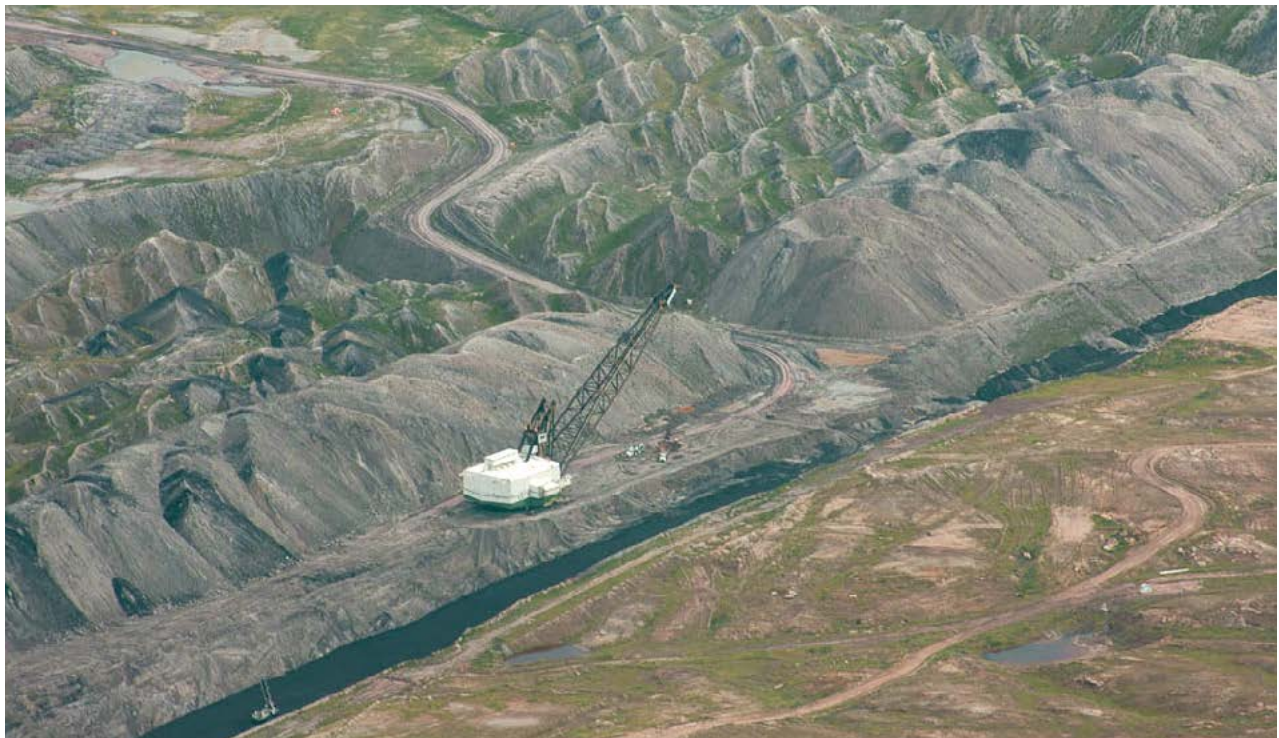
Figure 6 Aerial photograph of multiple rows of spoil ridges at Cloud Peak's Cordero Rojo Mine in Wyoming's Campbell County in July 2018. View is to the northeast. In the background, the spoil ridges are vegetated. This denotes the occurrence of one or more growing seasons since that land was mined, and it was not yet reclaimed at the time of the photo.
